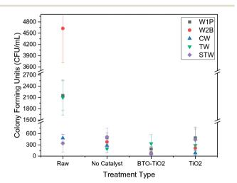
Fig. 4 Plot showing the average colony counts for all water sources after 3 hours of each treatment type, compared with the raw, untreated water.
