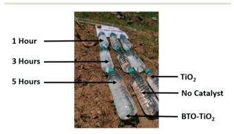
Fig. 3 Image to illustrate the way in which the bottles were set-up throughout the investigation.
