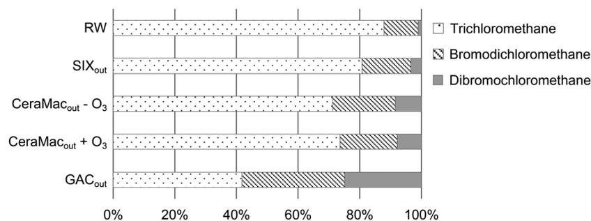
Fig. 7 Percentage of different THM species formed during high-dose chlorination after each stage of the pilot treatment (RW,  $\text{SIX}_{\text{out}}$ ,  $\text{CeraMac}_{\text{out}} - \text{O}_3$ ,  $\text{CeraMac}_{\text{out}} + \text{O}_3$ ,  $\text{GAC}_{\text{out}}$ ), based on the average of two replicates (experiment 3). Tribromomethane was not detected.
