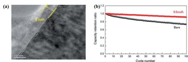
Fig. 14 (a) TEM image of a cross section of a 0.5 mol% LZO coated NCA particle. The right hand (dark) side corresponds to NCA; (b) cycle characteristics of bare and 0.5 mol% LZO coated NCA at  $25^\circ\text{C}$ . Reproduced with permission.<sup>121</sup> Copyright© 2013, Elsevier B.V.
