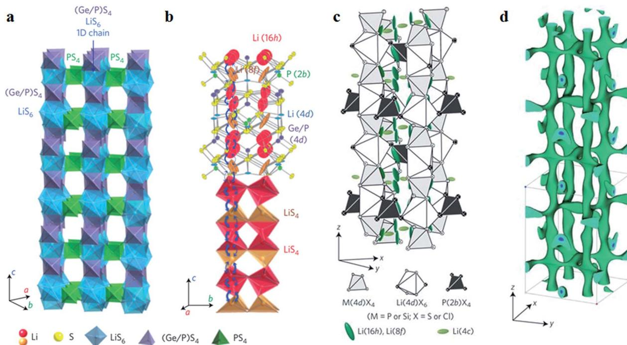
Fig. 4 (a) Framework structure of LGPS; (b)  $\text{Li}^+$  conduction pathways in LGPS; (c) crystal structure of  $\text{Li}_{9.54}\text{Si}_{1.74}\text{P}_{1.44}\text{S}_{11.7}\text{Cl}_{0.3}$ ; (d) nuclear distributions of Li atoms in  $\text{Li}_{9.54}\text{Si}_{1.74}\text{P}_{1.44}\text{S}_{11.7}\text{Cl}_{0.3}$  at 25 °C. Reproduced with permission.<sup>37,38</sup> Copyright© (2011, 2016), Springer Nature.
