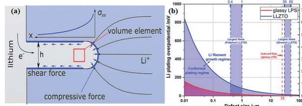
Fig. 21 (a) The effect of stress accumulation on lithium growth; (b) inverse square root dependence of Li plating over-potential and crack-extension stress ( $\sigma_{0,\text{max}}$ ) on defect size of glassy LPS and LLZTO. Reproduced with permission.<sup>165</sup> Copyright© 2017, John Wiley and Sons.
