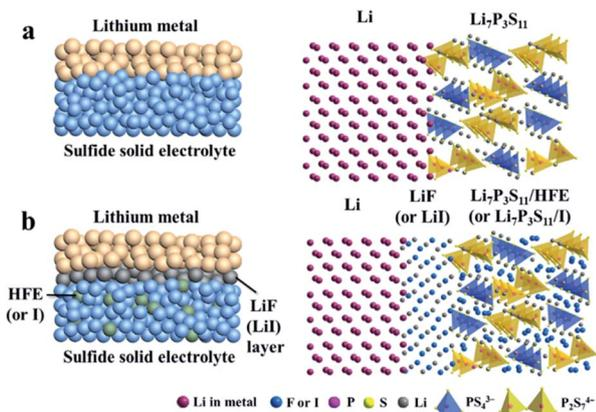
Fig. 19 Schematic diagrams of (a)  $\text{Li}/\text{Li}_7\text{P}_3\text{S}_{11}$  interface of ASSLIBs and (b) modified interface with a uniform thin LiF (or LiI) interphase layer and HFE (or I solution) infiltrated sulfide electrolyte. Reprinted with permission.<sup>164</sup> Copyright© 2018, Elsevier B.V.
