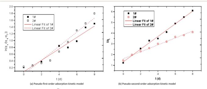
Fig. 12 Kinetic curves of adsorption Mn<sup>2+</sup> by immobilized particles. 1# is modified corncob fixed SRB sludge particles, 2# is unmodified corn cob fixed SRB sludge particles.
