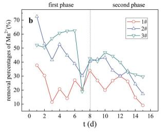
Fig. 7 (a)  $Mn^{2+}$  residual concentration in Columns 1, 2, 3 (b) The removal percentage of  $Mn^{2+}$  in Columns 1, 2, 3. Influent is the  $Mn^{2+}$ concentration in influent water of AMD. 1#, 2# and 3# in (a) are the residual Mn<sup>2+</sup> concentration in AMD after repairing AMD with Column 1, Column 2 and Column 3 respectively. 1#, 2# and 3# in (b) are the removal percentage of Mn<sup>2+</sup> in AMD by the three dynamic columns corresponding to (a) respectively
