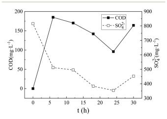
Fig. 2 COD release and  $SO_4^{2-}$  residual concentration at different modification time. The NaOH concentration was 5%, the  $H_2O_2$  concentration was 1.5%.
