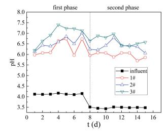
Fig. 9 The changes of pH in Columns 1, 2, 3. Influent is the pH value in influent water of AMD. 1#, 2# and 3# are the pH value in AMD after repairing AMD with Column 1, Column 2 and Column 3 respectively.
