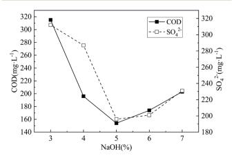
Fig. 3 COD release and  ${\rm SO_4}^{2-}$  residual concentration under different NaOH concentration. The  ${\rm H_2O_2}$  concentration was 1.5%.the modification time was 24 h.
