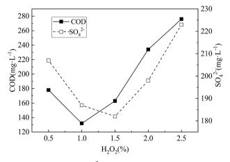
Fig. 4 COD release and  $SO_4^{2-}$  residual concentration under different  $H_2O_2$  concentration. The NaOH concentration was 5%, the modification time was 24 h.
