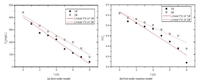
Fig. 10 Kinetic curves of  $SO_4^{2-}$  reduction by immobilized particles. 1# is modified corncob fixed SRB sludge particles, 2# is unmodified corn cob fixed SRB sludge particles.
