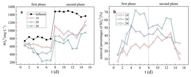
Fig. 5 (a)  $SO_4^2$  residual concentration in Columns 1, 2, 3 (b) Removal percentage of  $SO_4^2$  in Columns 1, 2, 3. Influent is the  $SO_4^2$ concentration in influent water of AMD. 1#, 2# and 3# in (a) are the residual  $SO_4^{2-}$  concentration in AMD after repairing AMD with Column 1, Column 2 and Column 3 respectively. 1#, 2# and 3# in (b) are the removal percentage of  $SO_4^{2-}$  in AMD by the three dynamic columns corresponding to (a) respectively.
