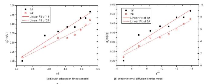
Fig. 11 Kinetic curves of adsorption  $Fe^{2+}$  by immobilized particles. 1# is modified corncob fixed SRB sludge particles, 2# is unmodified corn cob fixed SRB sludge particles.
