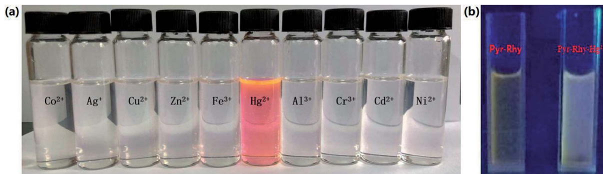
Fig. 4 (a) Colorimetric performance of sensor Pyr-Rhy (10 \mu\text{M} ) upon addition of different metal ions (1.0 equiv.) in DMSO/H 2 O (1/1, v/v) solution; (b) color change induced upon addition of Hg 2+ under 365 nm UV lamp.
