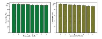
Fig. 8 Reusability test of the present  $Fe_3O_4$ -Ag nanocomposite as a catalyst for the reduction of 4-NP (a) and 2-NA (b) for eight consecutive cycles.
