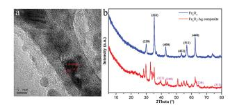
Fig. 4 HRTEM image of Ag nanowires (a) and XRD patterns of the  ${\rm Fe_3O_4-Ag}$  nanocomposite (b).
