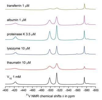
Fig. 3 51V NMR spectra showing interactions of 1 mM aqueous solutions of  $V_{10}$  with model proteins under given concentrations in 0.1 M MES buffer, 0.5 M NaCl at pH = 5.8. The black line represents the spectrum of the referent  $V_{10}Co$  and the coloured lines show the spectra of solutions of  $V_{10}Co$  in the presence of different proteins at given concentrations
