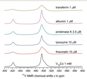
Fig. 4  $\,^{51}\!\text{V}$  NMR spectra showing interactions of 1 mM aqueous solutions of  $V_{10}Co$  with model proteins under given concentrations in 0.1 M MES buffer, 0.5 M NaCl at pH = 5.8. The black line represents the spectrum of the referent  $V_{10}Co$  and the coloured lines show the spectra of solutions of  $V_{10}Co$  in the presence of different proteins at given concentrations.
