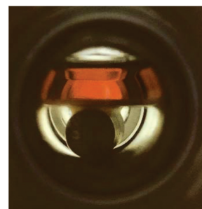
Fig. 2 Observed catalyst partitioning for 2 in a typical experiment prior to addition of reaction gases. (Top: orange n -decane phase containing the catalyst; bottom: colorless MeOH phase with 1,2-dimethyl-imidazole (1,2-DMI).
