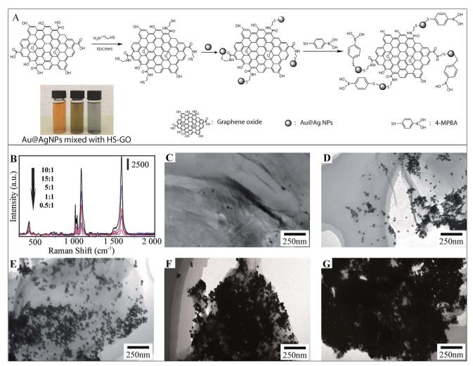
Fig. 2 (A) Schematic illustration of the fabrication of SERS tags and photographs of Ag@AuNPs (left), Au@AgNPs mixed with HS-GO for 5 min (middle) and 10 min (right); (B) SERS enhancement of Au@Aq-GO nanocomposites prepared with different Au@AqNPs/GO ratios (mL: mq): from 0.5:1 to 15:1. Raman spectra from the 4-MPBA adsorbed on the Au@Aq-GO surface; (C-G) TEM images of Au@Aq-GO nanocomposites prepared with different Au@AgNPs/GO ratios (mL: mg): 0.5:1 (C), 1:1 (D), 5:1 (E), 10:1 (F) and 15:1 (G).
