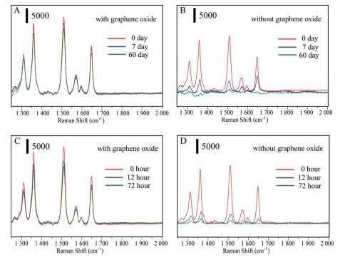
Fig. 3 (A and B) SERS spectra of  $10^{-9}$  R6G mixed with Au@AgNPs and Au@Ag-GO nanocomposites, both of which are stored at 4 °C for 0, 7 and 60 days; (C and D) SERS spectra of  $10^{-9}$  M R6G mixed with Au@AgNPs and Au@Ag-GO nanocomposites, both of which are placed in sunlight for 0, 12, and 72 hours.
