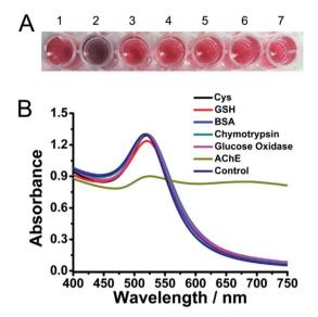
Fig. 4 Selectivity of the AChE sensor. (A) The color change of the solution in response to different species including biothiols and proteins that may exist in human body. (1) Control; (2) AChE; (3) Cys; (4) GSH; (5) BSA; (6) chymotrypsin; (7) glucose Oxidase. (B) Absorption curves of the solutions in (A). The final concentration of each biothiol was 0.1 mM and the enzymes was 1 U mL $^{-1}$ .
