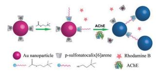
Fig. 1 System for detection of AChE activity based on RhB-p-SC<sub>6</sub>A-AuNPs aggregation and RhB release induced by the competitive host—guest interaction between p-SC<sub>6</sub>A-AuNPs and RhB/quaternary ammonium group.
