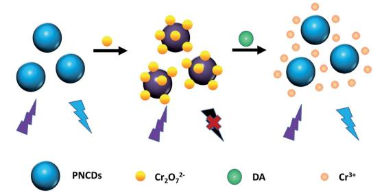
Scheme 1 Diagrammatical explanation of fluorescence mechanism for Cr(vi) and DA based on IFE of PNCDs.
