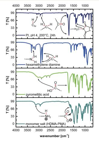
Fig. 2 ATR-FTIR spectra of PI6 and monomers. From top to bottom: PI6, HMDA, PMA, and monomer salt. Mode assignments are illustrated by molecule drawings
