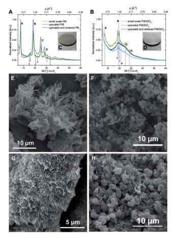
Fig. 7 PI6 and PI6/SiO $_2$  upscaling and sintering. (A) and (B) Comparison of the diffractograms of small scale synthesis, upscaled synthesis and material after sintering (PI6: (A) PI6/SiO $_2$ : (B)). (C) and (D) Photographs of the PI6 (C), and the PI6/SiO $_2$  pellet from sintering. (E)–(H) SEM images of upscaled PI6 before (E) and after (G) sintering, and of upscaled PI6/SiO $_2$  before (F) and after (H) sintering.
