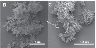
Fig. 5 Pl6/SiO<sub>2</sub> hybrids prepared from HMDA, PMA and TEOS. (A) Diffractograms of Pl6/SiO<sub>2</sub> prepared using different  $n_{\rm TEOS}$ ; amorphous backgrounds are highlighted. (B) and (C) SEM images of Pl6/SiO<sub>2</sub> at  $n_{\rm TEOS}=1.5$  mmol; SiO<sub>2</sub> nanoparticles (B) coexist with Pl6 ribbons (C).
