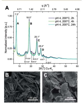
Fig. 3 Crystallinity of hydrothermally prepared PI6. (A) PXRD pattern of PI6 prepared at 200 °C and pH = 4 at  $t_R$  = 2 h (dark blue); 4 h (green) and 24 h (turquoise). Reflections are labelled (A)–(J) with annotated scattering angles  $2\theta$  (Cu–K $_{\alpha}$ ). (B) SEM image of PI6 synthesized at 200 °C and pH = 4 for 24 h. (C) SEM image of PI6 synthesized at 200 °C and pH = 1 for 24 h.
