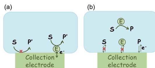
Fig. 1 Illustration of two possible enzyme detection methods *via* the nano-impact technique. (a) The enzyme collides with the electrode with which it undergoes direct electron transfer. (b) The catalytic reaction of the enzyme occurs in solution and the product is detected electrochemically.
