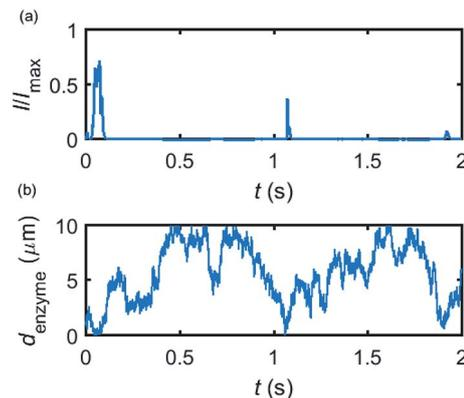
Fig. 6 Example of a simulated random walk current (a) and the corresponding pathway in the solution (b). The space, in which the enzyme moves freely, ranges from 5 nm to 10  $\mu\text{m}$ . Other simulation parameters are the same as applied in Fig. 5.
