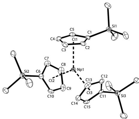
Fig. 5 Thermal ellipsoid drawing (50% probability for non-H atoms) of  $\text{NpCp}'_3$  in the solid state. H atoms omitted. Selected bond lengths [Å] and angles [°]: Np1–Ct1 2.485(2), Np1–Ct2 2.481(2), Np1–Ct3 2.479(2), Np1–C<sub>ar</sub> 2.734(6) to 2.786(4), Si1–(C1–C5) plane –0.382(8), Si2–(C6–C10) plane –0.109(8), Si3–(C11–C15) plane –0.169(8), Ct1–Np1–Ct2 119.86(8), Ct1–Np1–Ct3 120.46(7), Ct2–Np1–Ct3 119.06(8).
