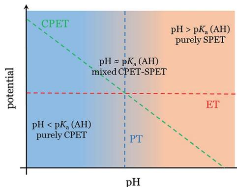
Fig. 2 Pourbaix diagram showing the thermodynamic equilibria of the CPET (green,  $\text{A} + \text{H}^+ + \text{e}^- \rightarrow \text{AH}$ ), ET (red,  $\text{A} + \text{e}^- \rightarrow \text{A}^-$ ) and PT (blue,  $\text{A}^- + \text{H}^+ \rightarrow \text{AH}$ ) steps.
