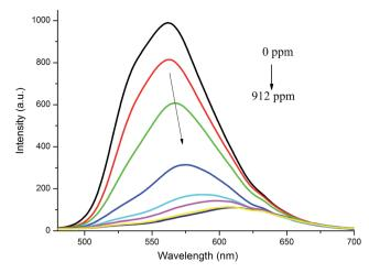
Fig. 7 Fluorescence spectra of TBM-based film upon exposure to different amounts of TFA vapor ( $\lambda_{ex} = 420$  nm).
