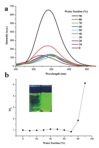
Fig. 3 (a) Fluorescence spectra of TBM in the mixtures of THF and water with different water fractions  $(f_w)$ ; (b) normalized fluorescence emission intensity of TBM in THF/water with different  $f_w$ . Concentration:  $1.0 \times 10^{-5}$  M;  $\lambda_{ex} = 410$  nm; inset is the fluorescence images of **TBM** in THF and THF/water ( $f_w = 90\%$ ) under 365 nm illumination.
