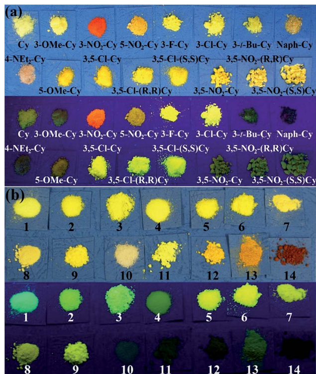
Fig. 3 Photographs (top: under room light, bottom: under 360 nm UV light) of Cys (a) and diPhs (b) 1 = diPh, 2 = 3-F-( R,R )-diPh, 3 = 3-F-( S,S )-diPh, 4 = 3-Cl-diPh, 5 = 3-Cl-( R,R )-diPh, 6 = 3-Cl-( S,S )-diPh, 7 = 3,5-Cl-diPh, 8 = 3,5-Cl-( R,R )-diPh, 9 = 3,5-Cl-( S,S )-diPh, 10 = 4-NEt 2 -diPh; 11 = Naph-diPh, 12 = 3-NO 2 -diPh, 13 = 5-NO 2 -diPh, 14 = 3,5-NO 2 -diPh) powders.
