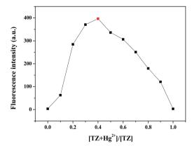
Fig. 8 Job plot examining the relationship between Z-3 and Hg<sup>2+</sup>.
