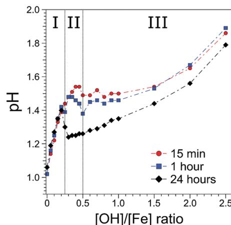
Fig. 1 Evolution of pH of  $0.75 \text{ M}$   $\text{FeCl}_3$  solutions as a function of  $h = [\text{OH}^-]/[\text{Fe}]$  ratio. Regions I–III correspond to the transitions from monomeric iron species to iron-oxo oligomers, and finally iron-oxo solid particles. Region I: oligomers with  $<1 \text{ nm}$  diameter. Region II: cylindrical particles. Region III: cylindrical particles and akaganeite formation.
