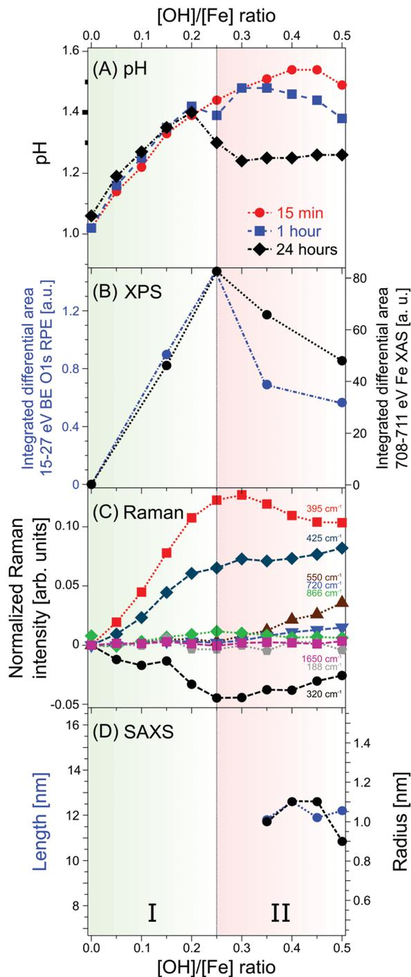
Fig. 4 Summary of trends from the different spectroscopic data as a function of the  $h = 0-0.5$  (A) pH. (B) Intensities of a and b PEY-XA bands for the O 1s and the Fe 2p edges, respectively. (C) Raman lines. (D) Particle lengths and radii from SAXS measurements.
