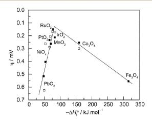
Fig. 3 Volcano plot showing activity for  $O_2$  production on metal oxide surfaces *versus* the enthalpy of transition of the oxide in acidic ( $\blacksquare$ ) and basic ( $\square$ ) solutions. Overpotential measured relative to 0.1 mA cm<sup>-2</sup> current density. Reprinted with permission.<sup>21</sup> Copyright 2010, American Chemical Society.
