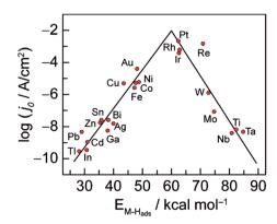
Fig. 2 Volcano curve for the HER on metal electrodes in acidic media. The log of the exchange current density  $j_0$  is plotted *versus* the M–H bond energy for each metal surface. Reprinted with permission.<sup>21</sup> Copyright 2010, American Chemical Society.
