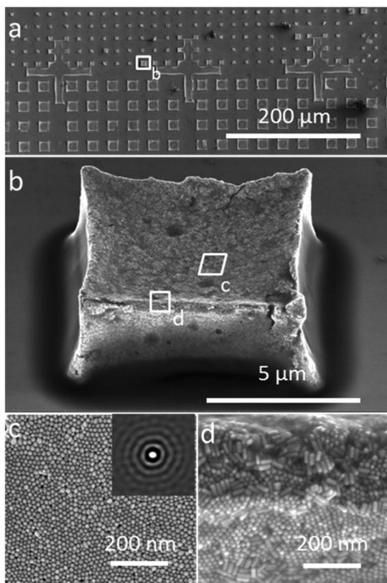
**Fig. 2** Hierarchically organized GNR supercrystals obtained by the PDMS driven self-assembly process. (a–d) SEM images taken at different magnifications of the supercrystal arrays deposited on Si (100). (c, d) The local hexagonal ordering of the nanorods was observed both on the top and at the edges of the supercrystals respectively. The inset in (c) shows autocorrelation analysis of the SEM image where up to five degrees of order can be distinguished.
