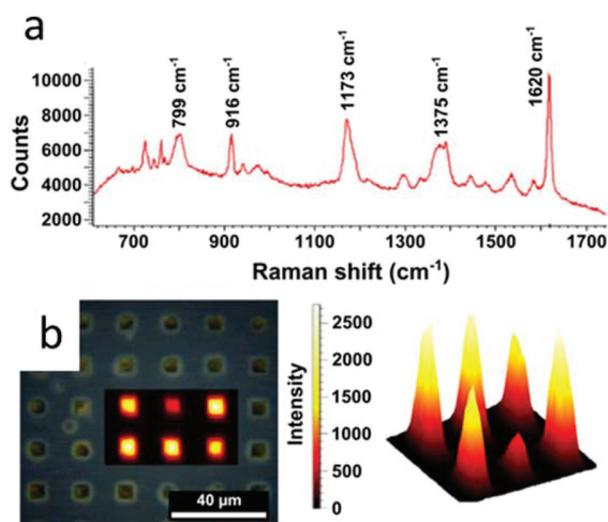
**Fig. 7** SERRS detection of Crystal Violet on an array of GNR supercrystals coated with mesoporous silica. (a) Typical SERRS spectra of CV measured on the supercrystals. (b) SERRS signal obtained by mapping the SERRS intensity of the crystal violet vibrational peak over  $1618\text{--}1632\text{ cm}^{-1}$ , as observed in a Raman microscope and reconstructed in three dimensions with intensity given as height.
