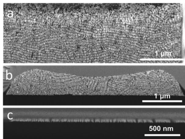
**Fig. 4** Effect of the gold nanorod concentration on the internal organization. SEM images of internal sections of GNR supercrystals after FIB cutting. GNR concentrations were  $375 \text{ mM}$  (a),  $37 \text{ mM}$  (b) and  $8.3 \text{ mM}$  (c).
