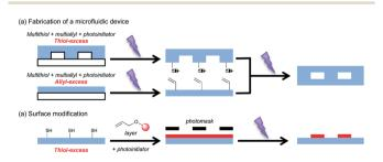
Fig. 11 An off-stoichiometric thiol-ene reaction was used to (a) fabricate a microfluidic device and for (b) surface modification. This example clearly shows the advantages of thiol-ene reactions that arise from their step-growth addition character and the availability of vast arrays of monomers that are used on combination with the control that light initiation affords. (Image adapted from ref. 98.)
