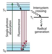
Fig. 2 Jablonski diagram. The excited singlet state  $(S_1)$  undergoes intersystem crossing (ISC) to a triplet state  $(T_1)$ , which leads to various photochemical reactions (e.g., radical generation as presented here). (Image adapted from ref. 16.)
