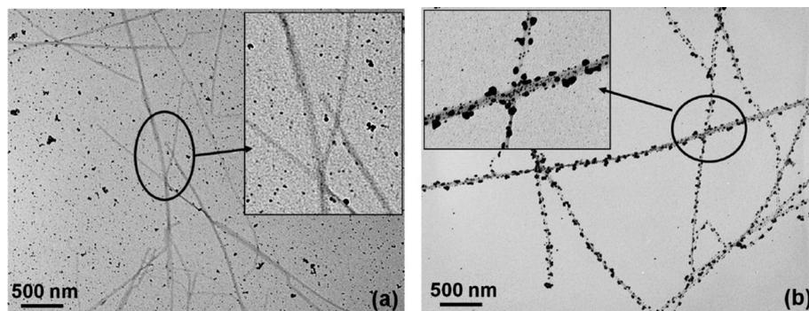
Fig. 3 TEM images of the AgNPs synthesis on tunicate NCC without CTAB (a) and with CTAB (b).<sup>90</sup> Reprinted with permission from S. Padalkar, J. Capadona, S. J. Rowan, C. Weder, Y. H. Won, L. A. Stanciu, R. J. Moon, Natural biopolymers: novel templates for the synthesis of nanostructures, *Langmuir*, 2010, 26(11), 8497–8502. Copyright 2014 American Chemical Society.
