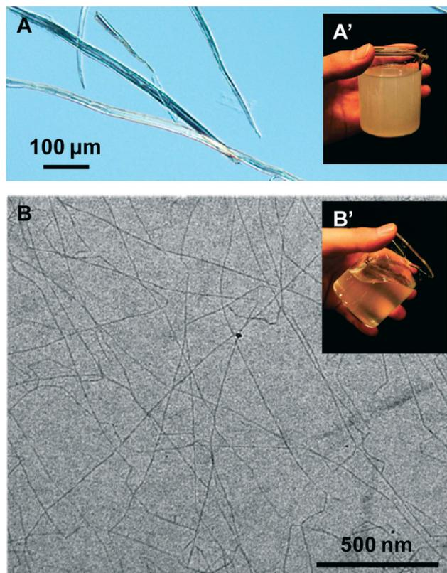
Fig. 1 a) Optical micrograph of TEMPO-oxidized cellulose fiber; b) TEM of the TEMPO-oxidized cellulose fiber.<sup>44</sup> Reprinted with permission from T. Saito, M. Hirota, N. Tamura, S. Kimura, H. Fukuzumi, L. Heux, A. Isogai, Individualization of nano-sized plant cellulose fibrils by direct surface carboxylation using TEMPO catalyst under neutral conditions, *Biomacromolecules*, 2009, 10(7), 1992–1996. Copyright 2014 American Chemical Society.
