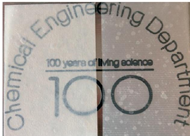
Fig. 2 Comparison of the transparent papers made from BC (left) and MFC (right).<sup>33</sup> Reprinted with permission from K. Y. Lee, T. Tammelin, K. Schultfer, H. Kiiskinen, J. Samela, A. Bismarck, High performance cellulose nanocomposites: comparing the reinforcing ability of bacterial cellulose and nanofibrillated cellulose, *ACS Appl. Mater. Interfaces*, 2012, 4(8), 4078–4086. Copyright 2014 American Chemical Society.
