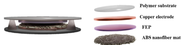
Fig. 2 Schematic representation of the ABS-based TENG.
