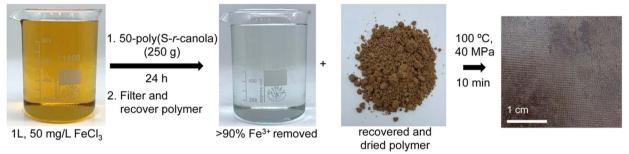
Fig. 13 (A) Reactive compression molding can be used to recycle the 50-poly(S-r-canola) material. (B) 50-poly(S-r-canola) can be used to remove Fe3+ from water and then repurposed to a new architecture via reactive compression molding. At these levels, the bound iron did not affect the reactive compression molding. Reproduced with permission from Chem. Eur. J. 2020, 26, 10035. Copyright 2025, John Wiley and Sons.
