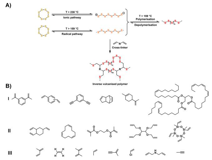
Fig. 3 (A) General scheme of IV via an ionic or radical reaction pathway. (B) Selection of reported cross-linkers suitable for IV. Group I: cross-linkers reactive without a catalyst in conventional IV; Group II: cross-linkers reactive with a catalyst; Group III: cross-linkers applicable in photoinduced IV.
