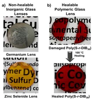
Fig. 11 (a) Damaged inorganic lenses (germanium lens (top) and zinc selenide lens (bottom)) that cannot be repaired for IR imaging. (b) Poly(S-r-DIB30) copolymer lens which is drastically damaged but repaired and functional by thermal annealing at 100 °C. Reproduced with permission from ACS Macro Lett. 2015, 4, 862-866. Under the Creative Commons public use license, CC-BY or CC-BY-NC-ND, American Chemical Society.
