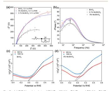
Fig. 5 (a) EIS Nyquist plots of BiVO<sub>4</sub>, 1% Nb: BiVO<sub>4</sub> and 5% Nb: BiVO<sub>4</sub> in 0.1 M K<sub>2</sub>SO<sub>4</sub> at different potentials and illumination (AM 1.5 G 100 mW cm<sup>-2</sup>). (b) Bode plots under the same conditions. Mott–Schottky plots of (c) BiVO<sub>4</sub> and (d) 5% Nb: BiVO<sub>4</sub> under illumination.
