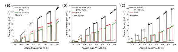
Fig. 7 Light-chopped linear sweep voltammograms of pristine  $BiVO_4$ , 1% and 5% Nb :  $BiVO_4$  films in (a) glycerin 10% v/v in  $K_2SO_4$  0.1 M, (b) crude glycerol 10% v/v in K<sub>2</sub>SO<sub>4</sub> 0.1 M and (c) raw flegmass with added 0.1 M K<sub>2</sub>SO<sub>4</sub>.
