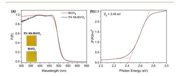
Fig. 4 (a) Diffuse reflectance spectra of BiVO $_4$  and 5% Nb : BiVO $_4$  films and (b) Tauc plot of BiVO $_4$ .
