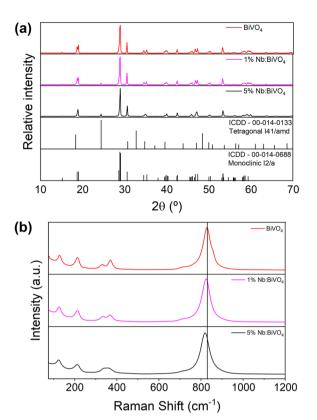
Fig. 1 (a) XRD patterns and (b) Raman spectra of pristine  $\rm BiVO_4$  and  $\rm Nb:BiVO_4$  samples.
