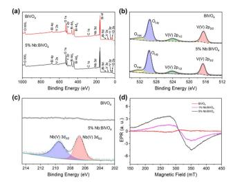
Fig. 2 (a) Survey spectra of  $BiVO_4$  and 5% Nb:  $BiVO_4$ ; (b) high-resolution XPS spectra of V 2p and O 1s; (c) high-resolution XPS spectra of Nb 3d; and (d) EPR spectra of the solid-state powder  $BiVO_4$ -based catalysts.
