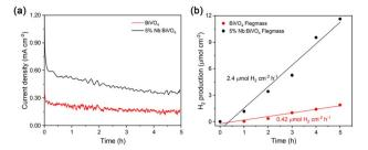
Fig. 9 (a) Chronoamperometry graphs of  $BiVO_4$  and 5% Nb:  $BiVO_4$  in raw flegmass, under 1.0 V vs. RHE and 100 mW cm² AM 1.5 G illumination. (b)  $H_2$  evolution from an average of 3 chronoamperometry experiments for  $BiVO_4$  and 5% Nb:  $BiVO_4$  photoanodes.
