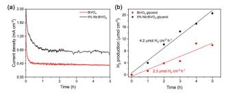
Fig. 8 (a) Chronoamperometry graphs of BiVO<sub>4</sub> and 5% Nb: BiVO<sub>4</sub> in crude glycerol 10%/v in K2SO4 0.1 M under 1.0 V vs. RHE and 100 mW cm<sup>2</sup> AM 1.5 G illumination. (b) H<sub>2</sub> evolution from an average of 3 chronoamperometry experiments for BiVO<sub>4</sub> and 5% Nb:BiVO<sub>4</sub> photoanodes
