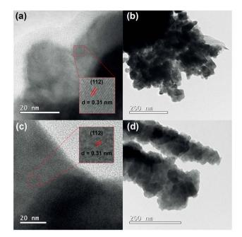
Fig. 3 HRTEM images of (a and b)  ${\rm BiVO_4}$  and (c and d) 5% Nb :  ${\rm BiVO_4}$  at different magnification levels.
