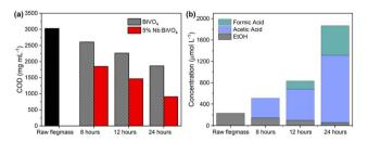
Fig. 10 (a) COD removal from flegmass after photoelectroforming experiments with different durations using the  $\rm BiVO_4$  and 5% Nb:  $\rm BiVO_4$  photoanodes. (b) HPLC results showing the variation in concentration of flegmass main oxidation products as a function of time during photoelectroforming experiments using 5% Nb:  $\rm BiVO_4$  photoanodes under simulated sunlight (AM 1.5 G 100 mW cm $^{-2}$ ) and 1.0 V vs. RHE applied bias.
