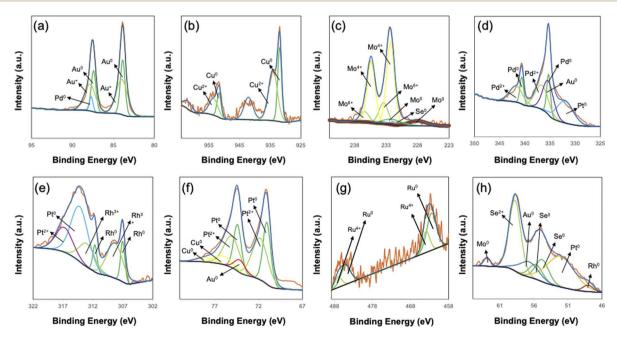
Fig. 4 XPS spectra of (a) Au 4f (overlapping with Pt 4d), (b) Cu 2p, (c) Mo 3d (overlapping with Se 3s), (d) Pd 3d (overlapping with Pt 4d and Au 4d), (e) Rh 3d (overlapping with Pt 4d), (f) Pt 4f (overlapping with Cu 3p and Au 5p), (g) Ru 3p, and (h) Se 2p (overlapping with Au 5p, Pt 5p, and Rh 4p) of the m-HEA film.
