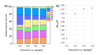
Fig. 5 (a) Relative molar compositions of elements (determined by ICP analysis, as shown in Table S3) and (b) corresponding mixed configuration entropy values ( $\Delta S_{\rm mix}$ ) at different deposition potentials.
