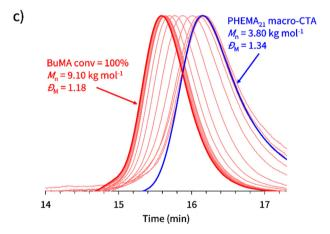
Fig. 1 Kinetic study for the RAFT emulsion polymerisation of BuMA, targeting a degree of polymerisation of 100, in [EMIM][EtOSO<sub>3</sub>] at 10% w/w solids using a PHEMA<sub>21</sub> macro-CTA: (a) BuMA conversion vs. time (blue circles) and semi-log kinetic (red squares); (b)  $M_n$  (blue circles) and  $D_M$ (red squares) vs. BuMA conversion; (c) DMF GPC chromatograms. GPC data were obtained against poly(methyl methacrylate) standards.
