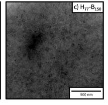
Fig. 4 TEM images obtained for 0.10% w/w emulsions of PHEMA-b-PBuMA block copolymers prepared in [EMIM][EtOSO3].
