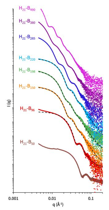
Fig. 5 Background-subtracted SAXS patterns recorded at 1.0% w/w for PHEMA $_{21}$ -b-PBuMA $_y$  spheres prepared via RAFT emulsion polymerisation, where dashed lines represent fits to the spherical micelle model. For clarity, data are offset on the y-axis by a factor of 10.
