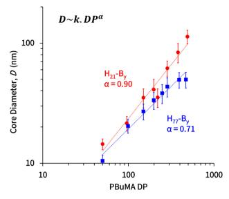
**Fig. 6** Relationship between core radius and target DP of the PBuMA block (y) for series of PHEMA<sub>21</sub>-b-PBuMA<sub>y</sub> (red circles) and PHEMA<sub>77</sub>-b-PBuMA<sub>y</sub> (blue squares) diblock copolymer spheres prepared via RAFT emulsion polymerisation of BuMA in [EMIM][EtOSO<sub>3</sub>] at 70 °C. The error bars represent the standard deviation of the diameter and  $\alpha$  is the scaling factor.
