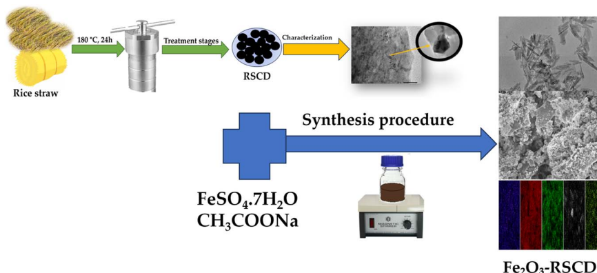
Scheme 1 The synthesis of Fe 2 O 3 -RSCD. 27
