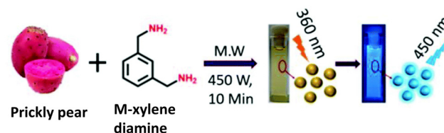
Fig. 6 Microwave-assisted synthesis of N-CDs from prickly pear and m -xylenediamine. 47 Copyright 2021, Royal Society of Chemistry.
