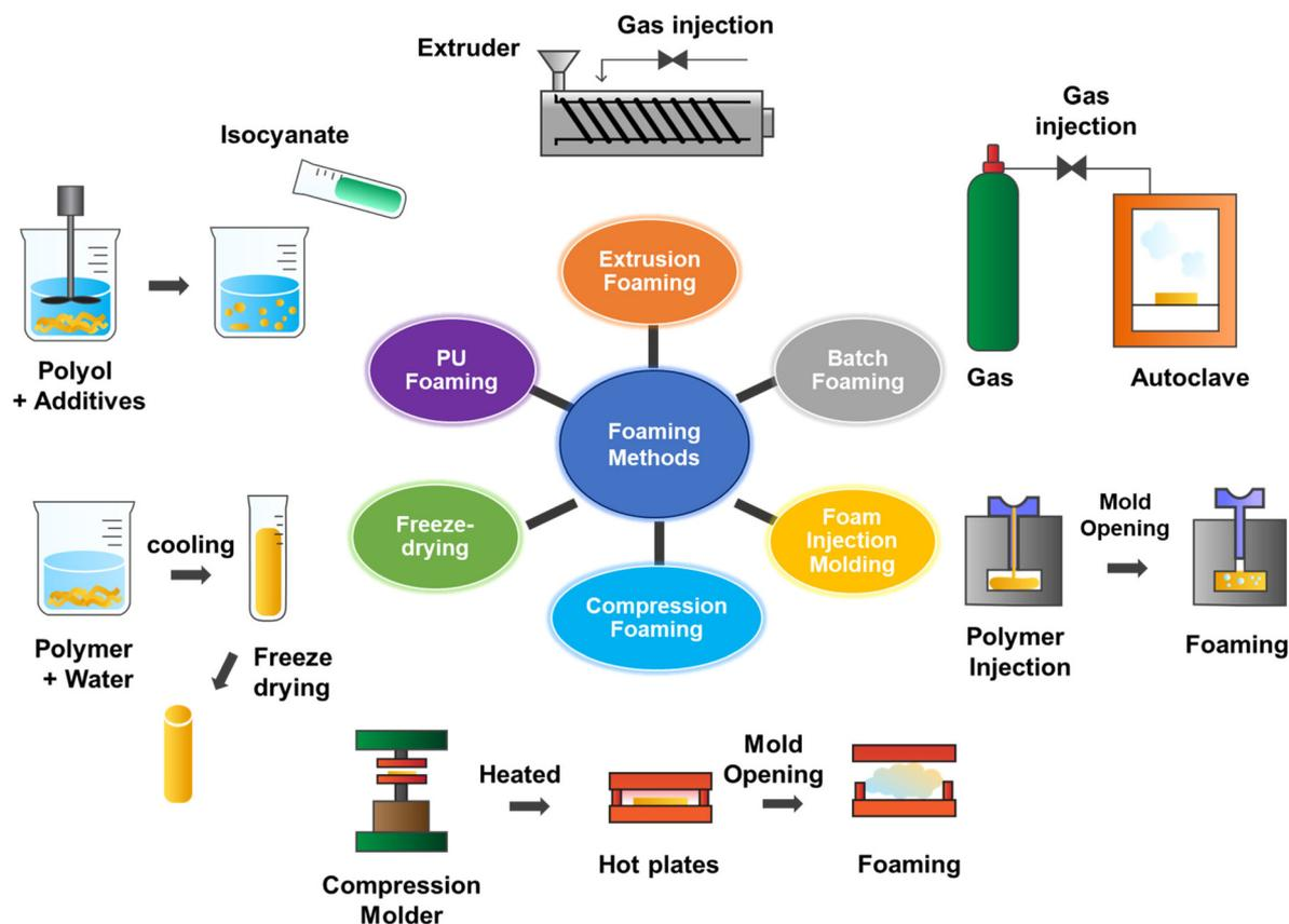
Fig. 6 Various foaming process methods to develop porous polymeric materials for oil spill cleanups.
