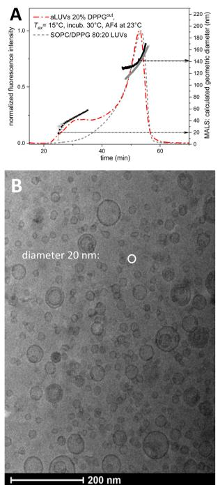
Fig. 4 Detection of small DVs in aLUV prepared at 15 °C after cyclodextrin removal and subsequent temperature increase as seen by AF4 (A) and cryo-transmission electron microscopy (cryo-TEM) (B). (A) The red dash-dot line (fluorescence signal, left axis) and black dots (MALS, right axis) represent a sample with 23 mol% DPPG in the outer leaflet after 30 min incubation at 35 °C, measured at 23 °C. The grey dashed curve (left axis) and
