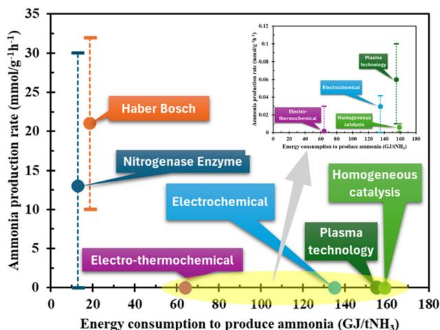
**Fig. 2** Illustration of energy consumption vs. production rate for several methods of nitrogen activation.<sup>12–15</sup>
