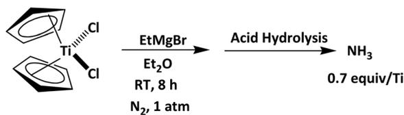
Scheme 1  $N_2$  activation by transition-metal complexes in moderate reaction operating conditions applying EtMgBr and  $Cp_2TiCl_2$ .<sup>102</sup>
