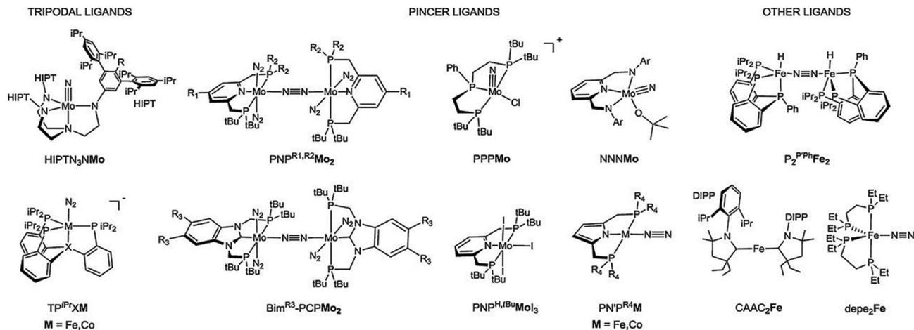
Fig. 12 Metal complexes for  $N_2$  activation through its reduction ( $X = C, B, Si$ ;  $Br, R = H$ ;  $R_1 = H, tBu, Me, OMe, Ph, Fc, Me_3Si$ ;  $Ad, R_2 = tBu$ ;  $R_3 = H, Me$ ;  $R_4 = tBu, Cy$ ;  $Ar = 2,6$ -diisopropylphenyl). Reproduced with permission from John Wiley & Sons. Copyright © 1999–2023 John Wiley & Sons.<sup>124</sup>
