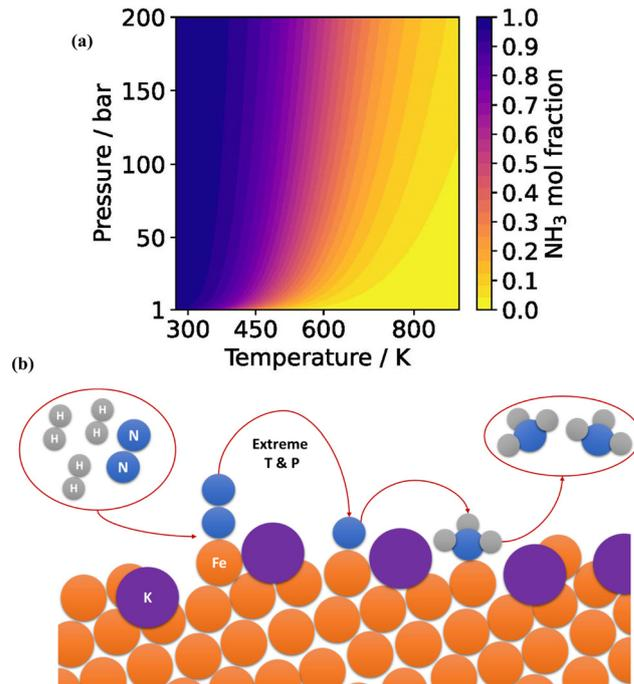
Fig. 3 (a) Thermodynamic equilibrium between  $\text{N}_2/\text{H}_2$  and  $\text{NH}_3$  (Haber–Bosch equilibrium); (b) animated illustration of the Haber–Bosch process, which occurs over a promoted iron catalyst at high temperature and pressure.
