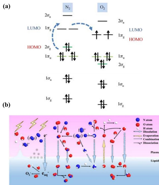
Fig. 15 (a) Scheme of molecular orbitals of  $N_2$  and  $O_2$ , reproduced from ref. 137 with permission from Springer Nature, Copyright © 2018, Higher Education Press and Springer-Verlag GmbH Germany, part of Springer Nature (b) schematic showing the fundamental processes in  $N_2$  plasma. Reproduced from ref. 138 with permission from Elsevier, © 2023 licensed via CC BY-NC-ND 4.0.
