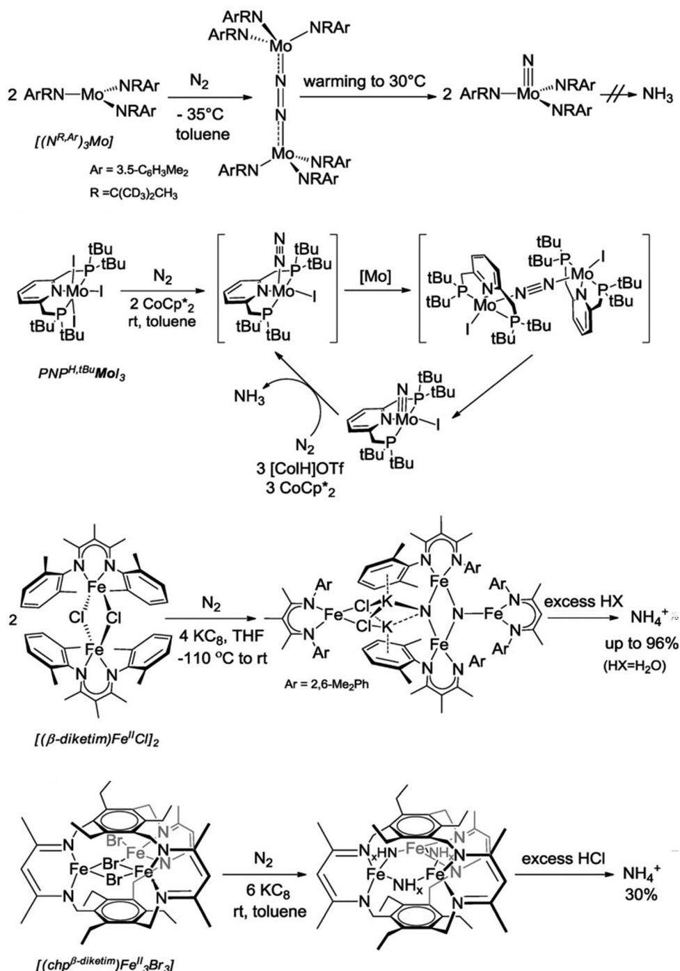
Fig. 11 Examples of dissociative mechanism for  $\text{N}_2$  activation. Reproduced with permission from John Wiley & Sons. Copyright © 1999–2023 John Wiley & Sons.<sup>124</sup>
