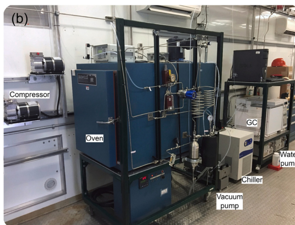
Fig. 16 Spiral wound module test rig for facilitated transport membrane assisted decarbonization; (a) schematic of the module's housing, (b) test setup (reproduced from ref. 197 with permission from Elsevier, copyright 2025).
