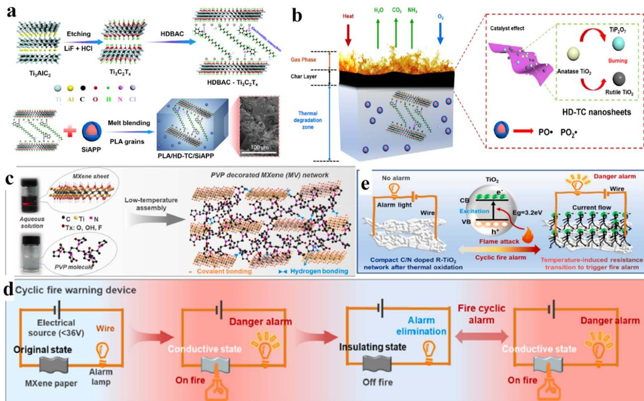
Fig. 25 (a) Synthetic scheme for HDBAC-Ti<sub>3</sub>C<sub>2</sub>T<sub>x</sub> and PLA/HD-TC/SIAPP. (b) Flame-retardant mechanism, reproduced from ref. 373 with permission from Elsevier, copyright 2022. (c) Low-temperature assembly for PVP-decorated MXene paper. (d) MXene paper-based fire-detecting sensing device (schematic). (e) Resistance transition mechanism of a C/N-doped TiO<sub>2</sub> network, reproduced from ref. 374 with permission from Elsevier, copyright 2022.
