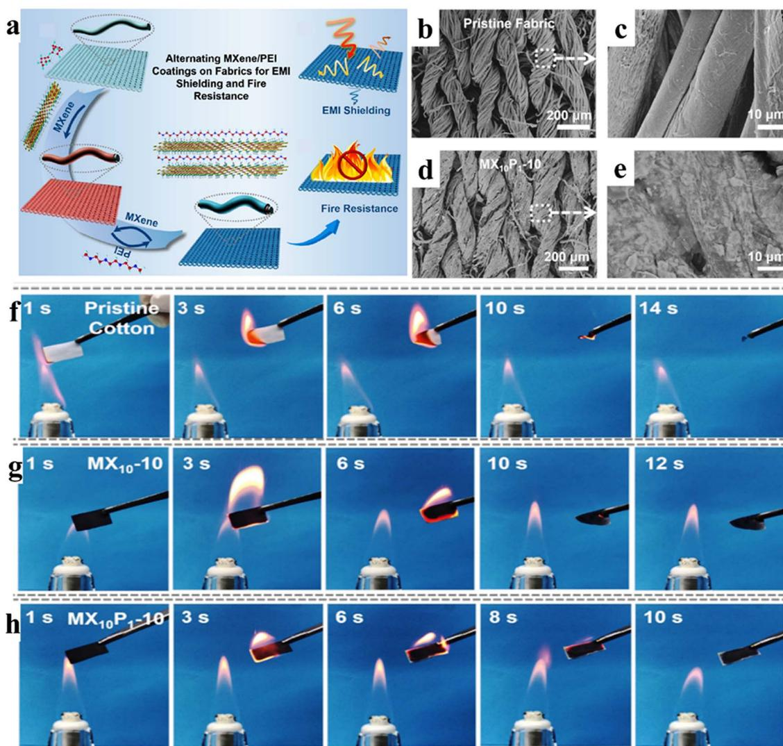
Fig. 24 (a) Assembly of a MXene/PEI-coated fabric. (b and c) SEM images of pristine cotton fabric. (d and e) SEM images of MX<sub>10</sub>P<sub>1</sub>-10. (f–h) Investigation of the fireproof properties of MX<sub>10</sub>-10 and MX<sub>10</sub>P<sub>1</sub>-10 fabrics, reproduced from ref. 370 with permission from American Chemical Society, copyright 2021.
