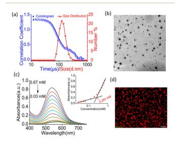
Fig. 1 (a) DLS profile of the self-assembled amphiphile (nanoaggregate). (b) TEM image of the nanoaggregate. (c) Nile-red absorption spectra by varying the concentration of LPA. Inset shows a plot of absorption intensity vs. concentration for CAC calculation (CAC = 263  $\mu$ M). (d) Fluorescence microscopy image of a Nile red-encapsulated nanoaggregate.
