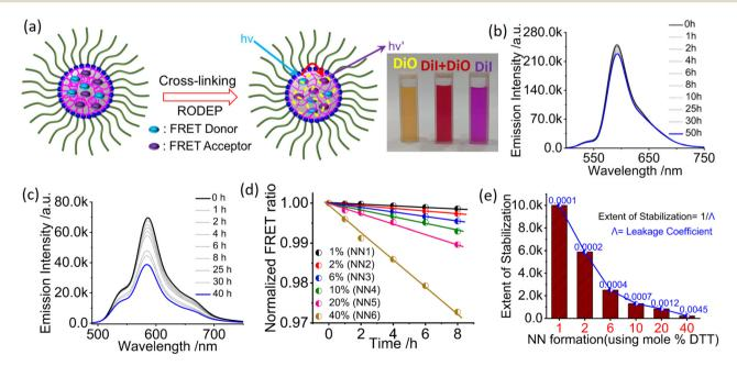
Fig. 8 (a) FRET by co-encapsulating Dil and DiO within the nanonetwork core (schematic). Images of the nanonetwork solution individually and loaded with a mixture of Dil and DiO. Monitoring of FRET by emission spectroscopy for the nanonetwork formed by (b) 1 mol% and (c) 40 mol% of DTT. (d) Calculation and comparison of the leakage coefficient of all nanonetworks from normalized FRET ratio vs. time plot. (e) Plot of leakage coefficient vs. various nanonetworks (NN1 to NN6).
