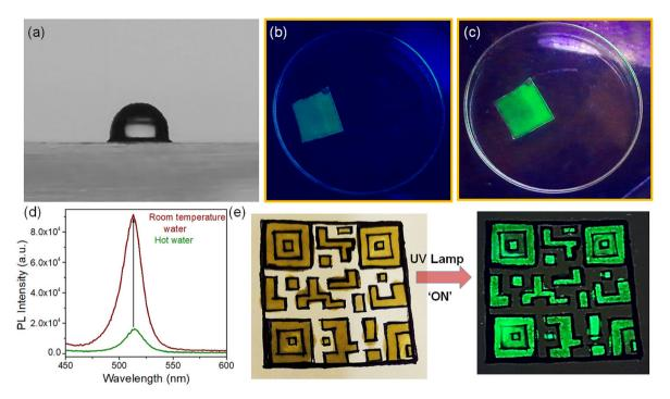
Fig. 6 (a) Study of the contact angle of a water droplet on a thin film of the fluorescent ink. Luminescence images of the film under exposure to a UV lamp at 365 nm (b) in hot water and (c) at room temperature. (d) Enhancement of PL intensity after exposing the film in hot water to room temperature water. (e) Anti-counterfeiting effect for a QR code which clearly shows the proper visibility under illumination with a UV lamp.
