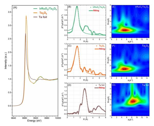
Fig. 4 (A) Ta L3-edge XANES spectra. FT-EXAFS spectra of (B) IrRuO<sub>x</sub>/Ta<sub>2</sub>O<sub>5</sub>, (C) standard Ta<sub>2</sub>O<sub>5</sub>, and (D) Ta foil. WT-EXAFS spectra of (E) IrRuO<sub>x</sub>/ Ta<sub>2</sub>O<sub>5</sub>, (F) standard Ta<sub>2</sub>O<sub>5</sub>, and (G) Ta foil.
