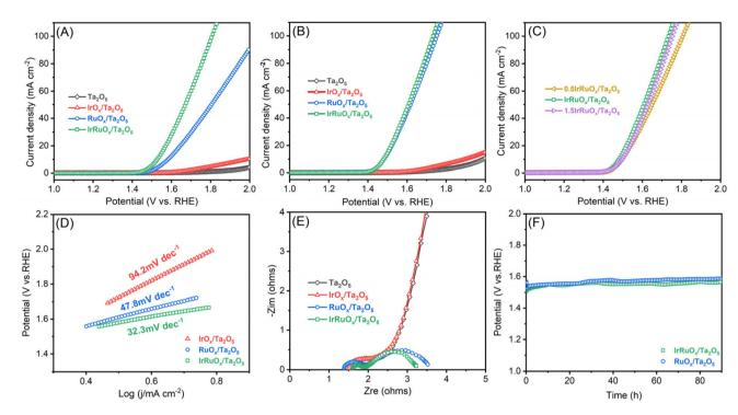
Fig. 5 OER LSV curves for the samples tested at (A) 0.4 mg cm<sup>-2</sup> and (B) 4 mg cm<sup>-2</sup>, and (C) different PGM/Ta ratios at 4 mg cm<sup>-2</sup> in 0.5 M H<sub>2</sub>SO<sub>4</sub>. (D) Tafel plots derived from OER voltammograms recorded at 4 mg cm<sup>-2</sup>. (E) EIS curves of the studied samples at 4 mg cm<sup>-2</sup>. (F) Chronopotentiometric curves of 4 mg cm $^{-2}$  IrRuO $_x$ /Ta $_2$ O $_5$  RuO $_x$ /Ta $_2$ O $_5$  at 10 A cm $^{-2}$  for 90 h.
