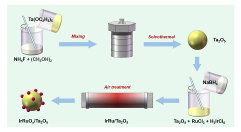
Scheme 1 Synthesis procedure for Ta<sub>2</sub>O<sub>5</sub> and IrRuO<sub>x</sub>/Ta<sub>2</sub>O<sub>5</sub>.
