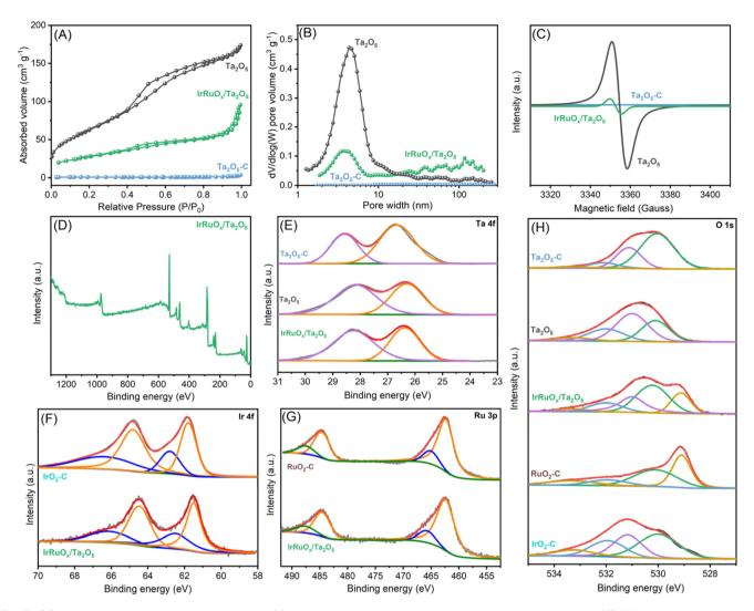
Fig. 3 (A) N<sub>2</sub> adsorption-desorption isotherms and (B) the resulting pore size distributions for the studied samples. (C) EPR spectra of the studied samples. (D) XPS full spectrum, (E) deconvoluted Ta 4f, (F) deconvoluted Ir 4f, (G) deconvoluted Ru 3p, and (H) deconvoluted O 1s spectra for the studied samples.
