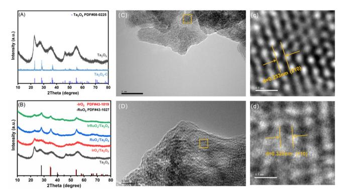
Fig. 1 (A) Comparison of XRD patterns between  $Ta_2O_5$  and  $Ta_2O_5$ -C. (B) Comparison of XRD patterns between  $Ta_2O_5$ ,  $IrO_x/Ta_2O_5$ ,  $RuO_x/Ta_2O_5$ , and  $IrRuO_x/Ta_2O_5$ . (C) TEM image and (c) HRTEM image of  $Ta_2O_5$ . (D) TEM image and (d) HRTEM image of  $Ta_2O_5$ .
