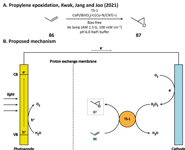
Fig. 13 Cathode-mediated *in situ* H<sub>2</sub>O<sub>2</sub> generation for propylene epoxidation.
