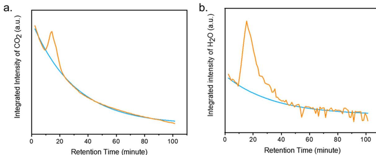
Fig. 7 (a) Integrated intensity of desorbed CO<sub>2</sub> (blue: background, orange: sample) and (b) integrated intensity of desorbed H<sub>2</sub>O (blue: background, orange: sample). Blue curve shows the background intensities of slow displacement of CO<sub>2</sub> and H<sub>2</sub>O from the carrier gas (He), while the orange curve indicates the integrated intensity of the adsorbed CO<sub>2</sub> and H<sub>2</sub>O from the chromatogram.
