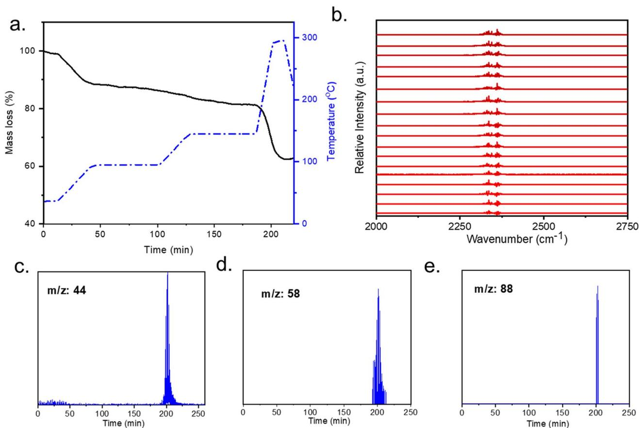
Fig. 4 TGA-FTIR-GCMS experiments on  $\text{mmen-Mg}_2(\text{dobpdc})$  with adsorbed  $\text{CO}_2$ : (a) thermogravimetric decomposition profile under humid He (black line); temperature ramp rate is shown in blue line; (b) FTIR spectra (0–50 min, 50–100 °C); characteristic  $\text{CO}_2$  was detected at 2360 and 2340  $\text{cm}^{-1}$ , each data was collected every 180 second. (c)–(e) gas chromatography mass spectra (GCMS) showing ions of released amine fragments.
