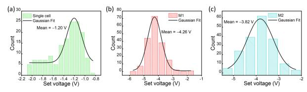
Fig. 3 Voltage distribution in the set process for (a) a single cell, (b) the first floor (M1), and (c) the second floor (M2).
