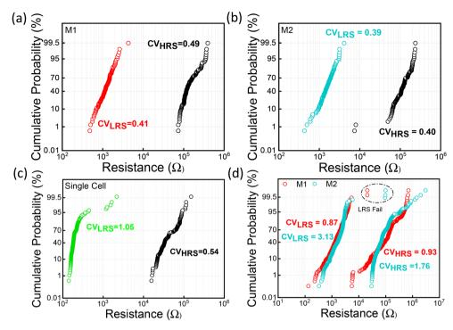
Fig. 4 Variation of the resistance parameters of four different cells within a device (a) on the first floor (M1) and (b) on the second floor (M2) from 30 consecutive cycles, and (c) five cells in a 2D single cell. (d) The resistance state the cumulative probability of fifteen devices of VRRAM (M1 and M2).
