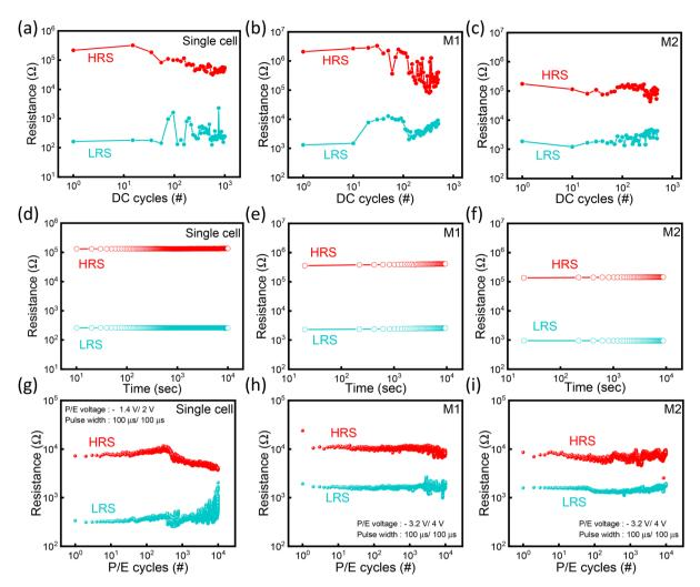
Fig. 5 Endurance characteristics of  $Pt/Ti/HfO_x/TiN-NCs/HfO_x/TiN$  for (a) a single cell, (b) the first floor (M1), and (c) the second floor (M2) in the HRS and LRS. Retention of three samples measured for 10 000 s: (d) a single cell, (e) M1, and (f) M2 in the HRS and LRS measured at 0.2 V. Pulse endurance: (g) a single cell, (h) M1, and (i) M2.
