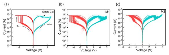
Fig. 2 /-V characteristics: (a) a single cell, (b) on the first floor (M1), and (c) on the second floor (M2) of VRRAM.
