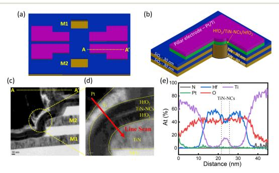
Fig. 1 3D schematic diagram of 4 × 2 × 2 vertical resistive random-access memory (VRRAM): (a) top view and (b) bird's eye view. (c) Cross-sectional TEM image and (d) enlarged switching area of Pt/Ti/HfO<sub>x</sub>/TiN-NCs/HfO<sub>x</sub>/TiN VRRAM (red line: EDS line scan). (e) Energy-dispersive spectroscopy (EDS) line analysis of VRRAM cells.
