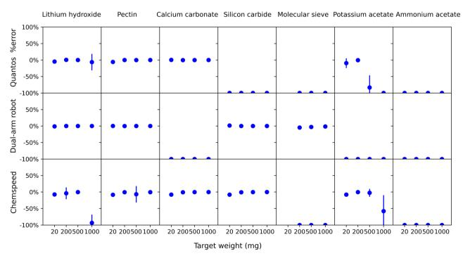
Fig. 6 Comparison between the different dispensing methods plotting average percentage dispensing error (see eqn (2)) with standard deviation for thirteen different solids with different target dispensing weights. Each row of sub-figures represents the data from a different dispensing platform, while each column represents a different solid. –100% dispensing indicates total failure to dispense the solid, most commonly because of a blockage.
