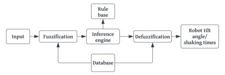
Fig. 5 Process for the fuzzy logic controller.
