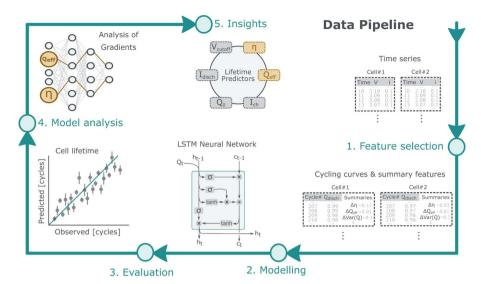
Fig. 1 Schematic overview of the prediction process.
