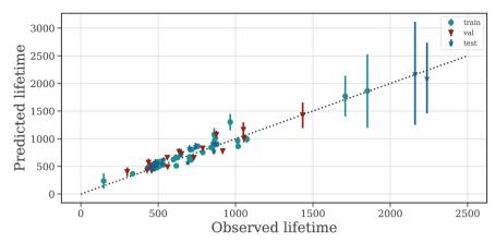
Fig. 2 LSTM ensemble prediction vs. ground truth based on 100 cycles. Error bars indicate SD.
