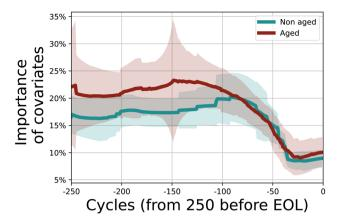
Fig. 9 Importance of in-cycle information for calendar-aged and non-calendar-aged batteries. The shaded area indicates one standard deviation in each direction
