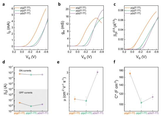
Fig. 2 (a) Transfer, (b) transconductance, and (c)  $I_D^{0.5}$  vs.  $V_G$  curves recorded for p(g2T-TT), p(p2T-TT), and p(b2T-TT). Comparison of the (d) on/off ratios, (e) electronic charge carrier mobilities, and (f) volumetric capacitances measured for the polymers.
