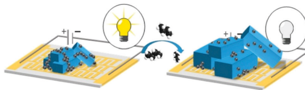
Fig. 5 Switchable MIL-53-carbon additive composite for CO 2 sensing. 25
