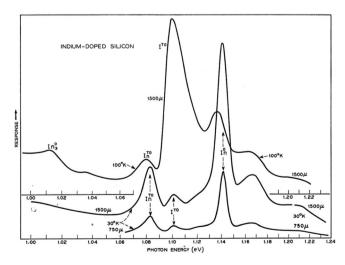
Fig. 4 30–100 K PL due to bound exciton recombination at indium atoms. <sup>16</sup> Reprinted with permission from P. J. Dean, J. R. Haynes and W. F. Flood, *Phys. Rev.*, **161**, 711–729, 1967. Copyright the American Physical Society, 1967.
