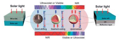
Fig. 20 Classes of spectral converters. Ala Reproduced with permission from C. X. Huang, S. Han, W. Huang and X. Liu, *Chem. Soc. Rev.*, 2013, **42**, 173–201. Copyright Royal Society of Chemistry.
