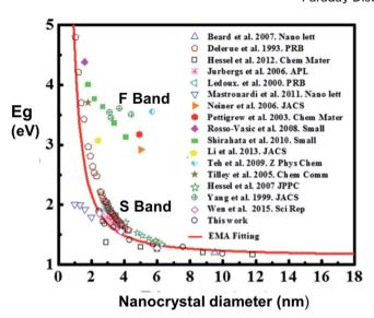
Fig. 13 Size dependence of photoluminescence for silicon quantum dots. Perinted with permission from X. Liu, Y. Zhang, T. Yu, X. Qiao, R. Gresback, X. Pi and D. Yang. Part. Syst. Charact., 33(1), 44–52, 2016. Copyright 2015, WILEY-VCH Verlag GmbH & Co. KGaA, Weinheim. Some of the featured studies reported F-band data rather than S-band data, as highlighted here.
