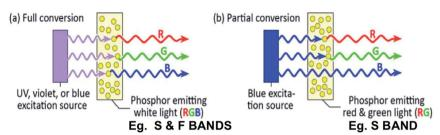
Fig. 22 White light generation using red, green or blue photoluminescent materials.<sup>429</sup> Adapted with permission from J. Cho, J. H. Park, J. K. Kim and E. F. Schubert, Laser Photonics. Rev., 2017, 11(2), 1600147. Copyright John Wiley & Sons.
