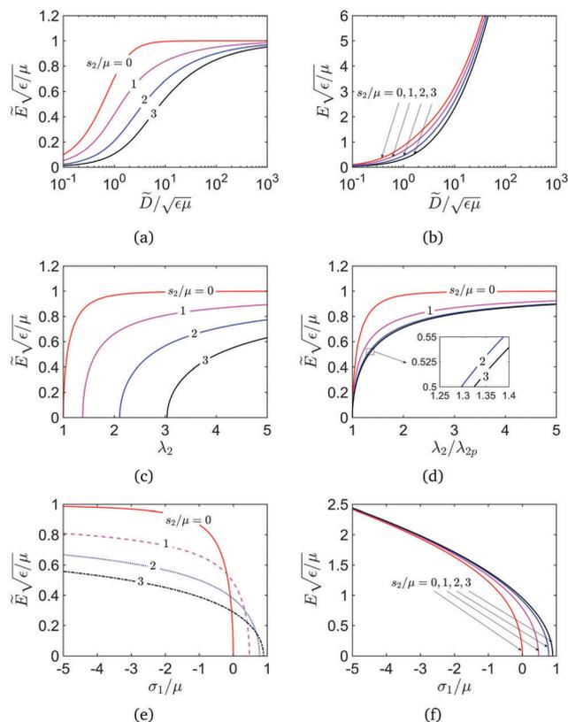
Fig. 2 Behavior of the neo-Hookean dielectric film at  $\lambda_1 = 1$  under various loads,  $s_2/\mu$ : (a) nominal electric displacement vs. nominal electric field, (b) nominal electric displacement vs. true electric field, (c) stretch  $\lambda_2$  vs. nominal electric field, (d) actuation stretch  $\lambda_2/\lambda_{2p}$  vs. nominal electric field, (e) true stress vs. nominal electric field, and (f) true stress vs. true electric field.
