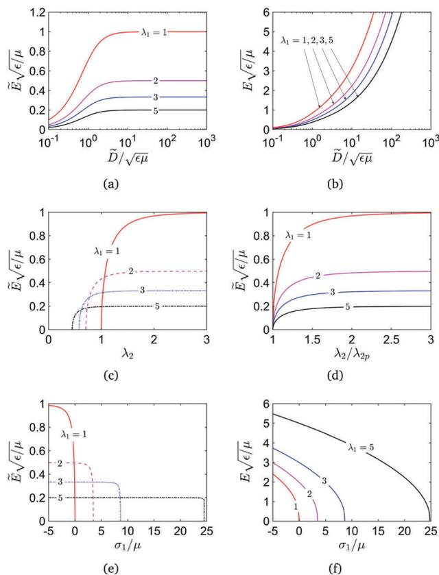
Fig. 3 Behavior of a neo-Hookean dielectric film at  $s_2 = 0$  under various stretches  $\lambda_1$ : (a) nominal electric displacement vs. nominal electric field, (b) nominal electric displacement vs. true electric field, (c) stretch  $\lambda_2$  vs. nominal electric field, (d) actuation stretch  $\lambda_2/\lambda_{2p}$  vs. nominal electric field, (e) true stress vs. nominal electric field, and (f) true stress vs. true electric field.
