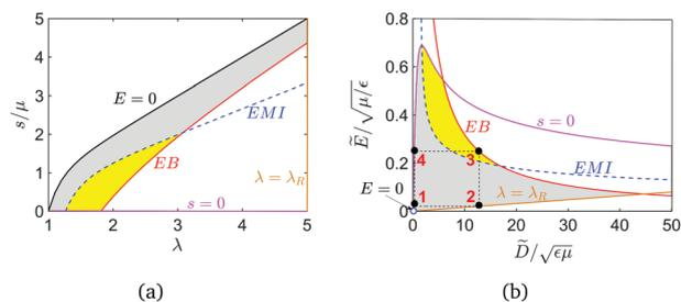
**Fig. 6** A thermodynamic state of the dielectric film is represented by (a) a point in the force–displacement plane or (b) a point in the voltage–charge plane. The equilibrium curve under the zero electric field is denoted as  $E = 0$ . Four modes of failure including EB, EMI, loss of tension  $s = 0$ , and rupture by stretch  $\lambda = \lambda_R$  are also plotted.
