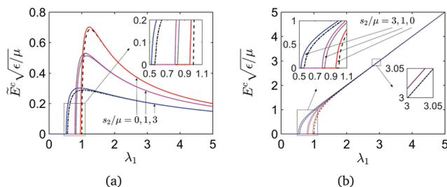
Fig. 4 Comparison of the loss of tension (dashed lines) and electrical buckling (solid lines) under several dead loads  $s_2/\mu$ . Effects of the stretch  $\lambda_1$  on (a) the critical nominal electric field and (b) the critical true electric field.
