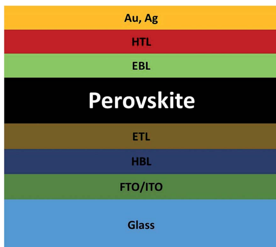
Fig. 1 Schematic of perovskite solar cell.
