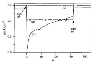
Fig. 1 Current density at -0.4~V measured on a  $0.5~\mu m$  thick  $Cu_2O$  electrode illuminated with 350 nm (5  $\times~10^{15}~s^{-1}~cm^{-2})$  in  $0.5~M~Na_2SO_4$  solution: (a) bubbled with air, (b) bubbled with Ar and (c) bubbled with Ar and with  $40~mM~MV^{2+}$  added to the solution.
