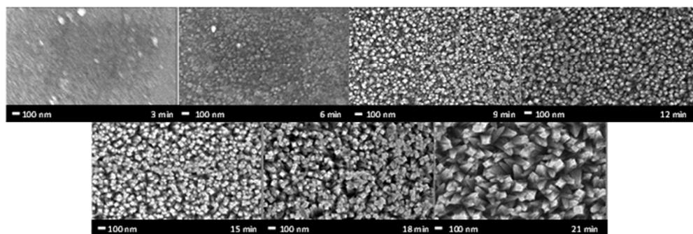
Figure 5: A time lapse of SEM images that represent 3, 6, 9, 12, 15, 18 and 21 minutes of the deposition process. It is evident that film formation occurs after 3 minutes with evidence of granular particulate matter forming with no overall order. After 9 minutes square structures start to appear and become progressively larger as the deposition process continues in time. Eventually the morphology resembles large monolithic square based pyramids after 21 minutes.
